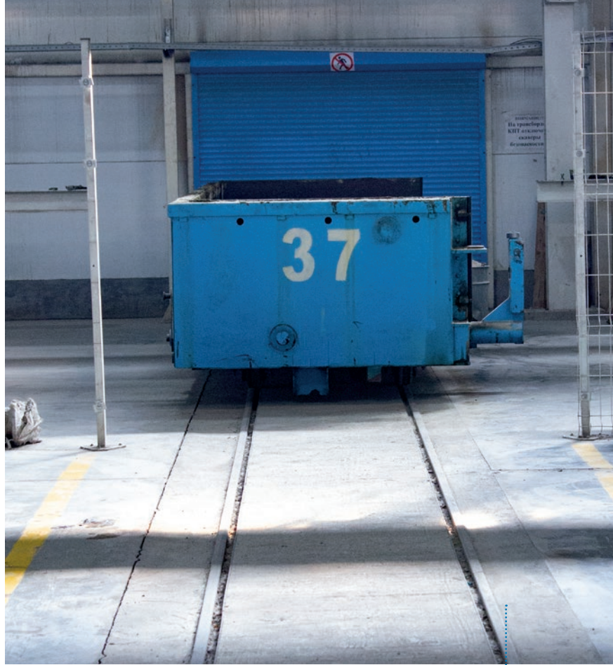
Mould before entry gate of fermentation area
