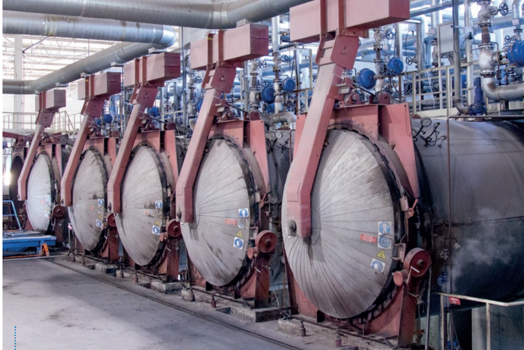
Each of the seven autoclaves in operation can receive a maximum of seven trolleys conveying three cakes each
