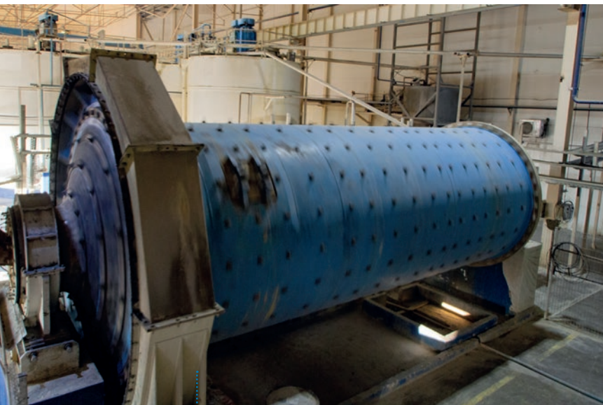
The Cemtech wet ball mill is controlled and monitored from an operating panel
